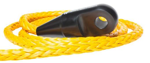
Synthetic ropes for crane applications have already been in development at WireCo for several years. The bright yellow rope, made by Lankhorst Ropes, consists of 12 braided outer strands made of the high-tech material Dyneema. The properties of these special fibres result in a breaking strength equal to a steel rope of the same thick-
